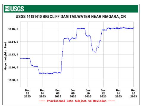
Figure 17. Gauge height (ft); below Big Cliff Dam.
