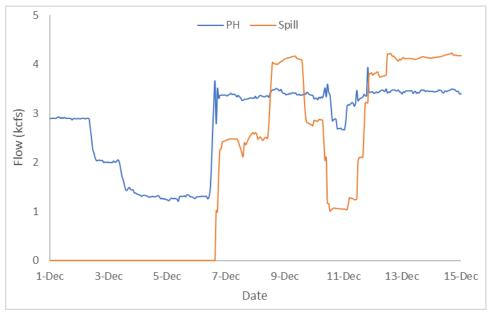
Figure 20. Hourly Flows PWR vs. Spill (Big Cliff Dam).
