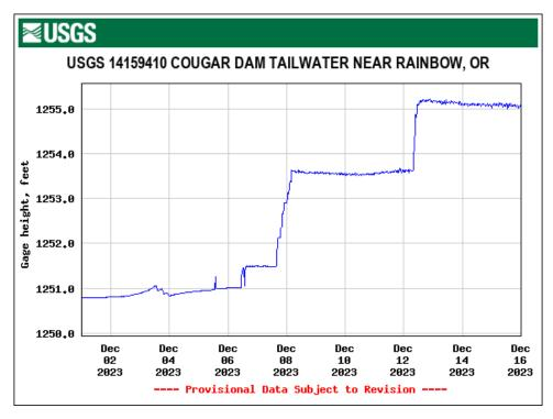
Figure 32. Gauge Height (feet); below Cougar Dam, South Fork McKenzie River.
