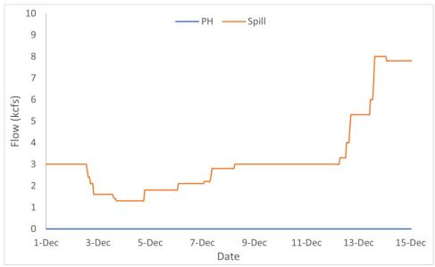
Figure 50. Hourly Flows PWR vs. Spill (Lookout Dam Tailrace).
