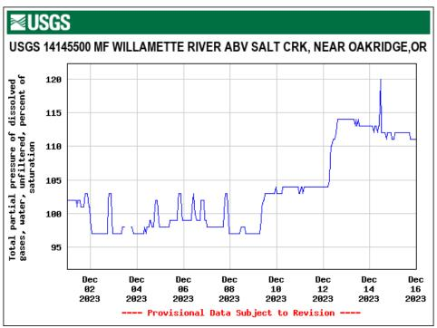
Figure 55. Total Dissolved Gas Saturation (%); below Hills Creek Dam – Middle Fork Willamette River.
