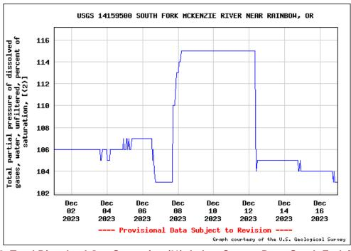
Figure 33. Total Dissolved Gas Saturation (%); below Cougar Dam, South Fork McKenzie River.
