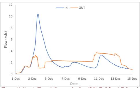
Figure 44. Hourly Flows Inflow vs. Outflow (RO) (Fall Creek Tailrace)
