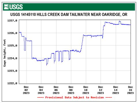
Figure 54. Gauge Height (feet); below Hills Creek Dam PWR - Middle Fork Willamette River.
